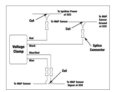
Figure 3 - Wiring Diagram & Wire Color Coding
